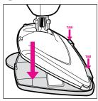
Attach carpet glide by placing unit under "tabs" and gently pushing down into place.
